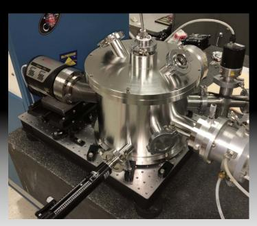
XUV soft x-ray and extreme ultraviolet spectrograph with flat field and diffraction gratings for 10 to 1500 eV now with Princeton Instruments PIXIS CCD detector and Lightfield® software
